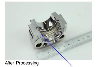
Corners of the mould have been protected during processing.
