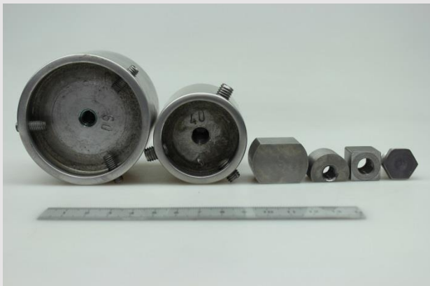
Special holders to cover the inside of the dies
