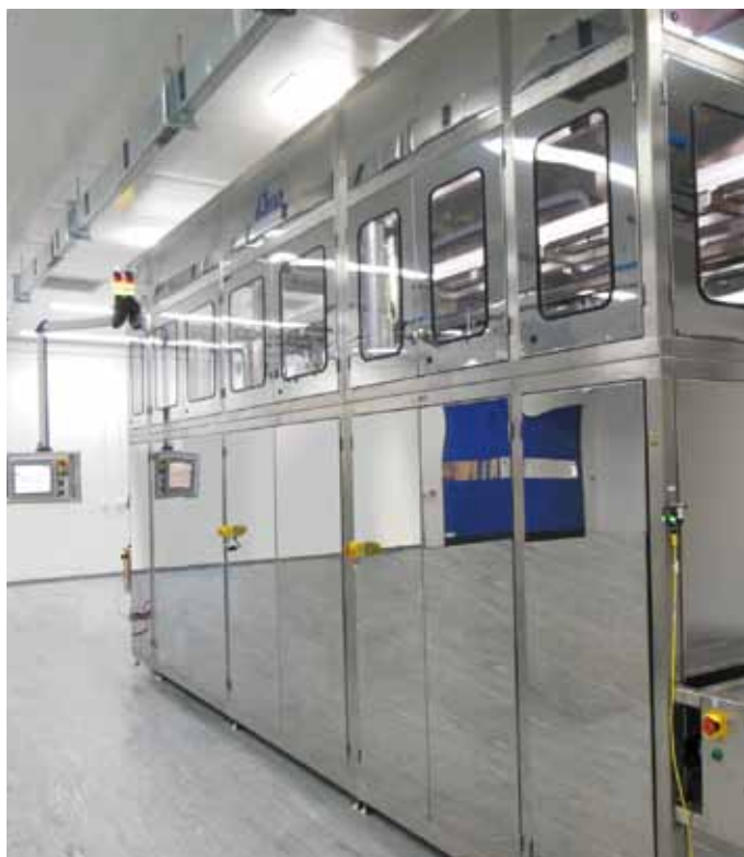
ELMA/ATEX 50-6-2-LRS 1 designed as multiple-chamber line for extraction and hydration
