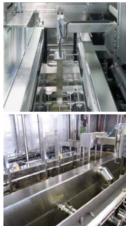
Basic chamber design with integrated process tanks, freeboard cooling system and technical extraction arranged above
