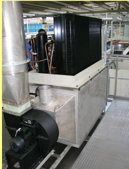
Pic. 3: Steam condenser, 3.500 m<sup>3</sup>/min, with integrated refrigerating machine, 25 kW refrigeration capacity
