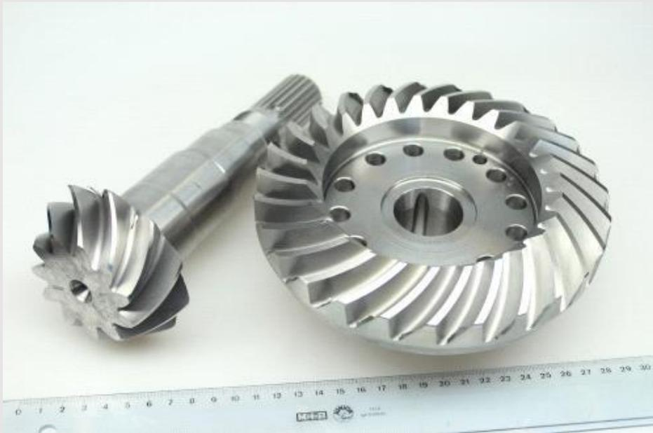
Drive shaft and bevel gear
