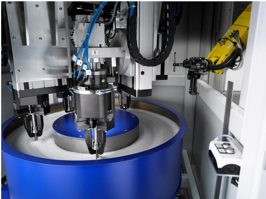
Fig. 1: Automatic loading of the SF machine
