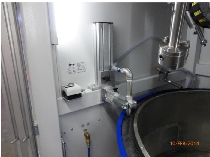
Fig. 4: Suction nozzle for extracting the waste water
