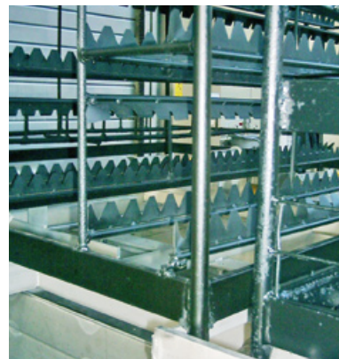
Painting rack before paint removal
