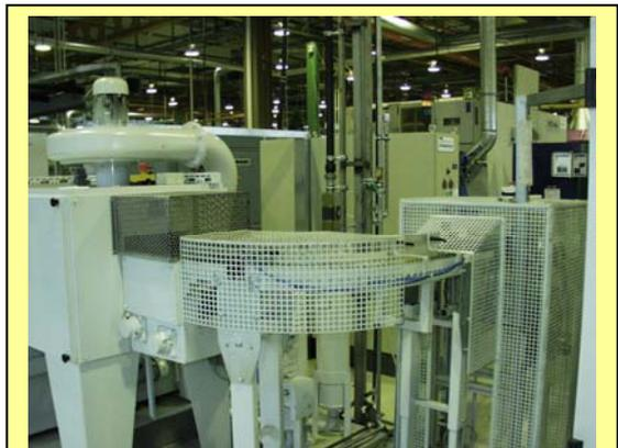
Pic. 5: Conveyor belt with turning station
