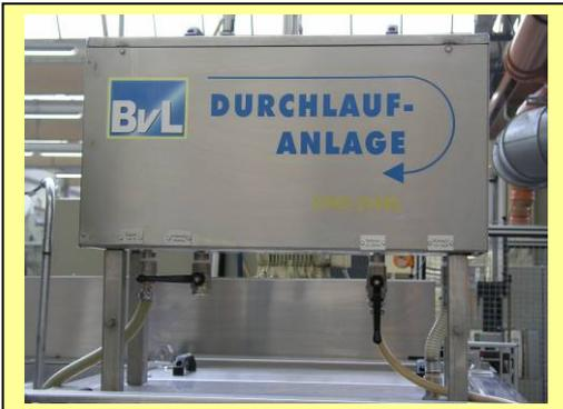
Pic. 1: Phase separator on the top of the unit for separation of oil
