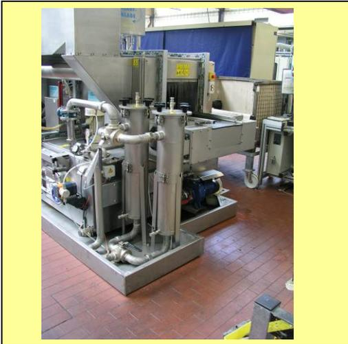
Pic. 3: Charging zone with pump for the tank rinsing
