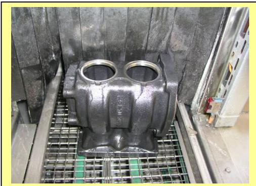
Pic. 5: Charging zone with sidewise adjustable guide and support rails
