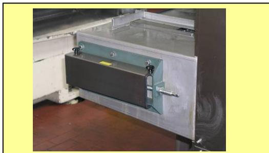
Pic. 6: Shielding of the clamping station
