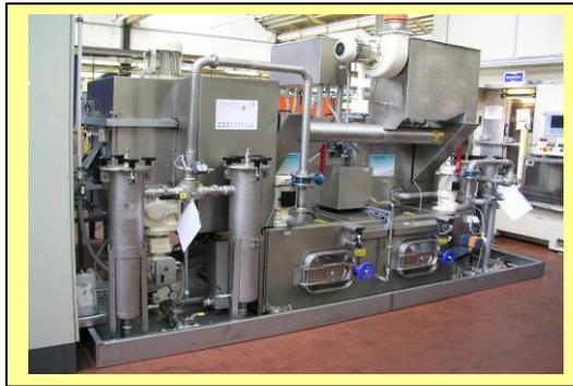
Pic. 2: View of the unit from the side with filter technology, blowing device, maintenance loops, condenser etc.
