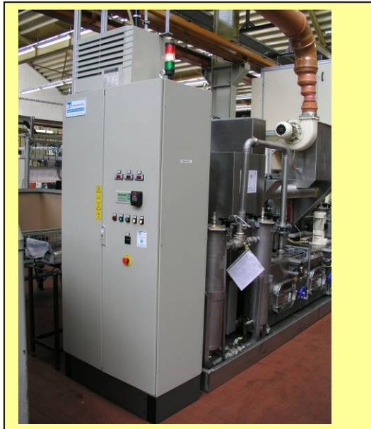
Pic. 4: Control cabinet with air conditioning and three-color signal lamp
