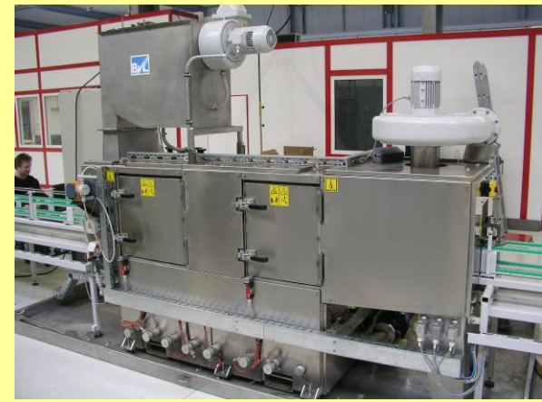
Pic. 2: Backside of the unit: big maintenance doors, steam condenser, blow-off fan, dosing pump
