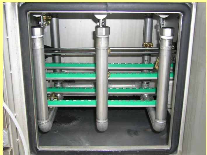
Pic. 4: Opened maintenance door with spraying system behind
