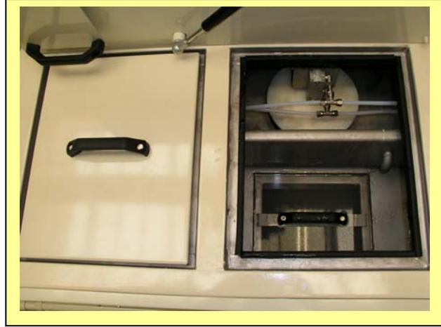
Pic. 2: removable tank covers. The return flow flaps and coarse filter boxes are arranged thereunder.
