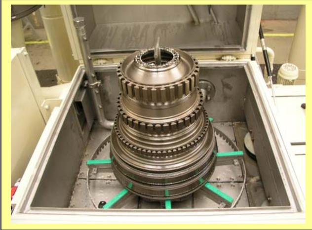
Pic. 1: Drum in the cleaning machine. By a snap closure the lance for internal cleaning can be removed quick and uncomplicated. For avoiding defects on the high-quality part the rotating assembly is equipped with green safety bars.
