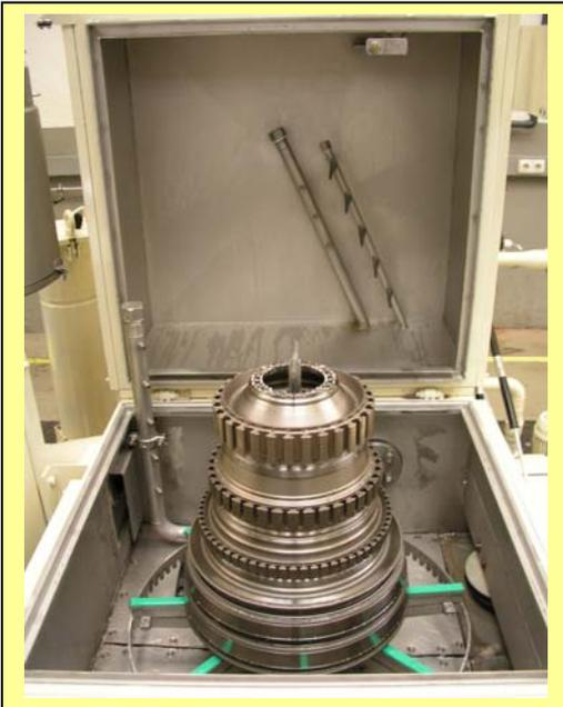
Pic. 3: Unit with opened cover and lance for the internal cleaning, blowing device, upper and lateral nozzle frame.
