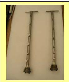
Pic. 6: nozzle lances for the internal cleaning
