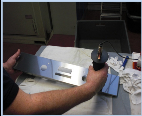
Pic. 1: Operator on checking a component; LED signalizes too high surface contamination
