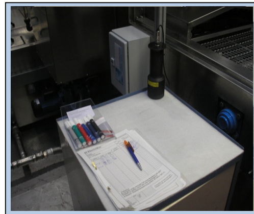
Pic. 4: Measuring booth for registration of the component cleanliness
