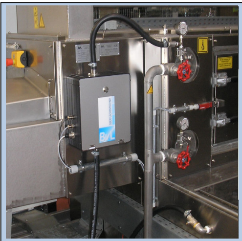
Pic. 3: Measuring cell for analysis of medium in the washing tank
